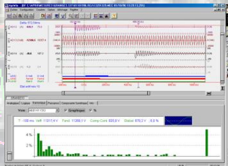
Analysis software (APRWIN) RMS values, power, harmonics, undervoltage, overvoltage ...
